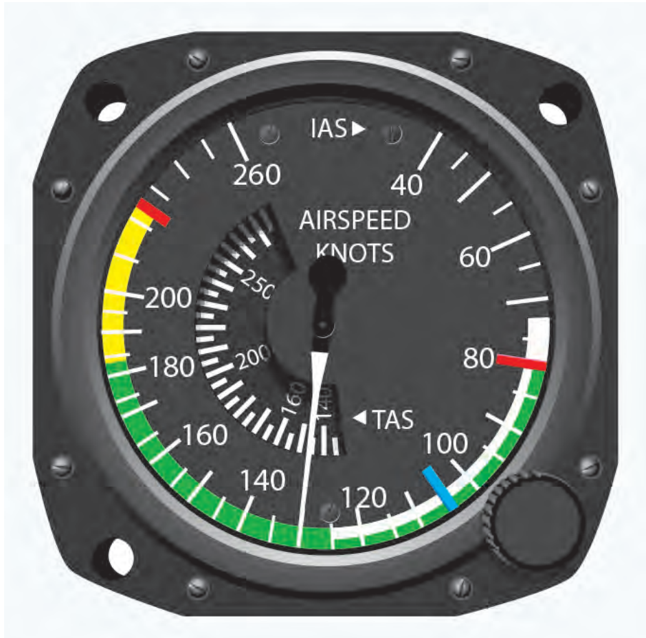
Figure 13-1. Airspeed indicator markings for a multiengine airplane
