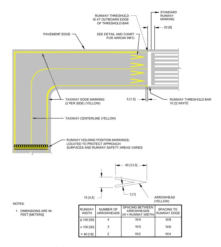
Figure 7. Marking for Aligned Taxiway with Runway Without a Displaced Threshold
