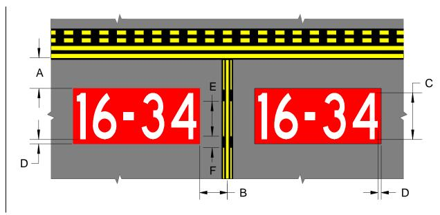
Figure C - 5. Surface Painted Holding Position Signs for Taxiway Widths Greater Than 35 Feet  $(10.5\ m)$
