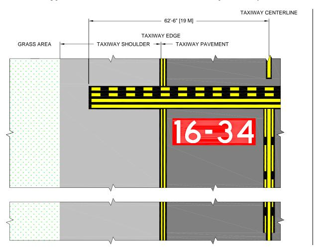
Figure C - 4. Enhanced Runway Holding Position Markings on Taxiways
