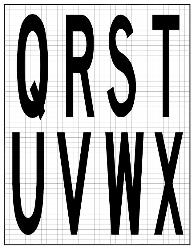
Figure A - 3. Pavement Markings QRSTUVWX
